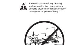
Leave enough slack in cable to allow for full range of vertical motion (19.3" / 49 cm). Failure to heed this warning may result in property damage and or personal injury.
