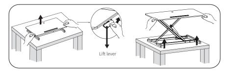
Loosen the lift lever and raise the tabletop at a suitable height according to your demands.
