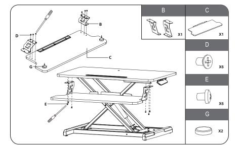
Install parts B under the keyboard plate. Then fasten the strews to mount the keyboard plate under the desktop.
